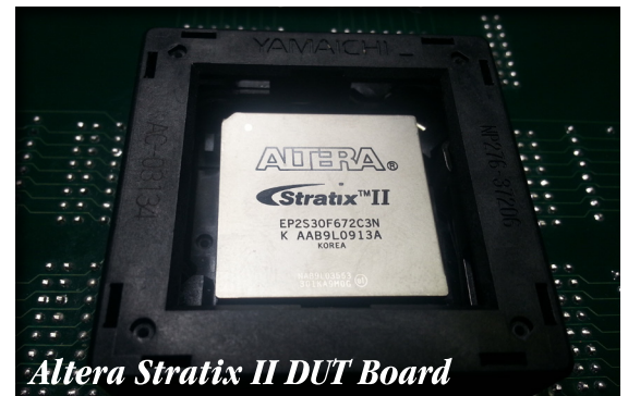
1517-Pin Custom DUT Board
